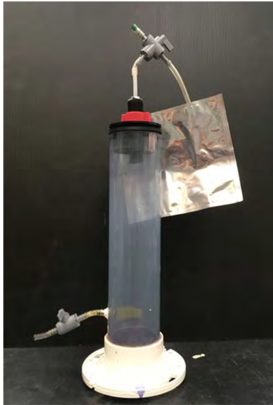
Figure 2-4 Laboratory Continuous Reactor and Multi-Foil Bag to Collect Biogas
