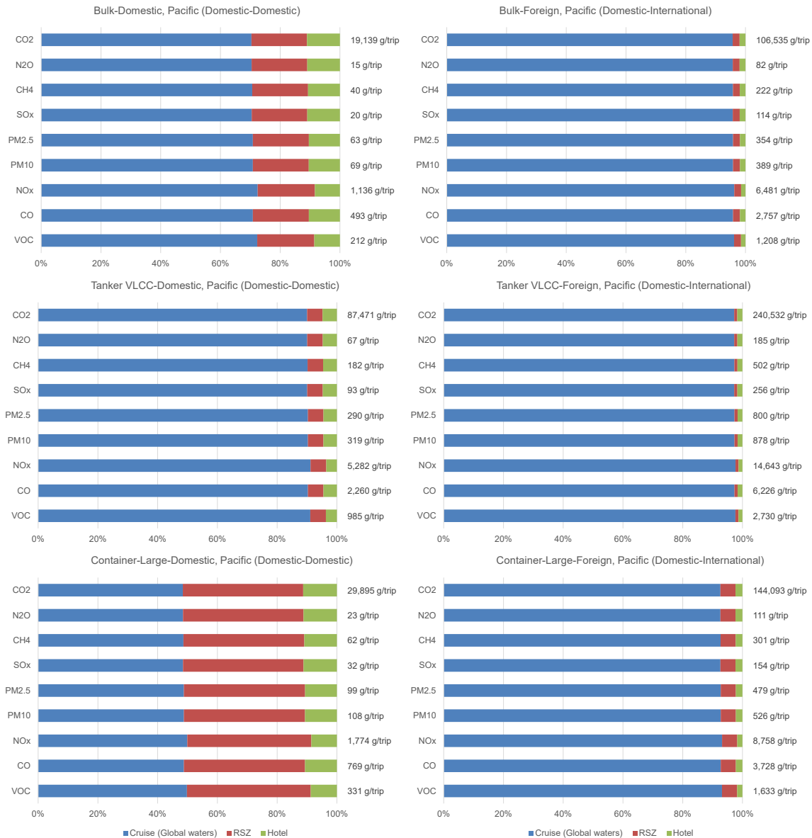
Figure 11. WTH GHG and CAP emissions, for example, trip conditions using FT-marine diesel. These are for three marine vessel types (bulk, tanker, and container) for two trip conditions in the Pacific (domestic and international). The numbers presented right-hand side of each chart represent total emissions during the trip.
