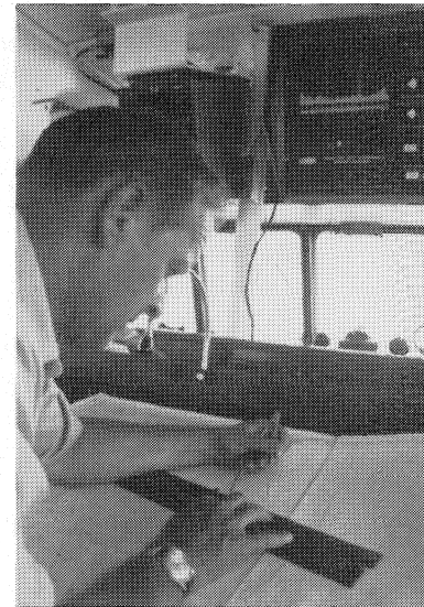
(Above) Anti-stranding sonar system, developed under MarAd's R&D program, gives warning of underwater obstructions and shoals in ship's path by use of long range and highly directional sound beams
