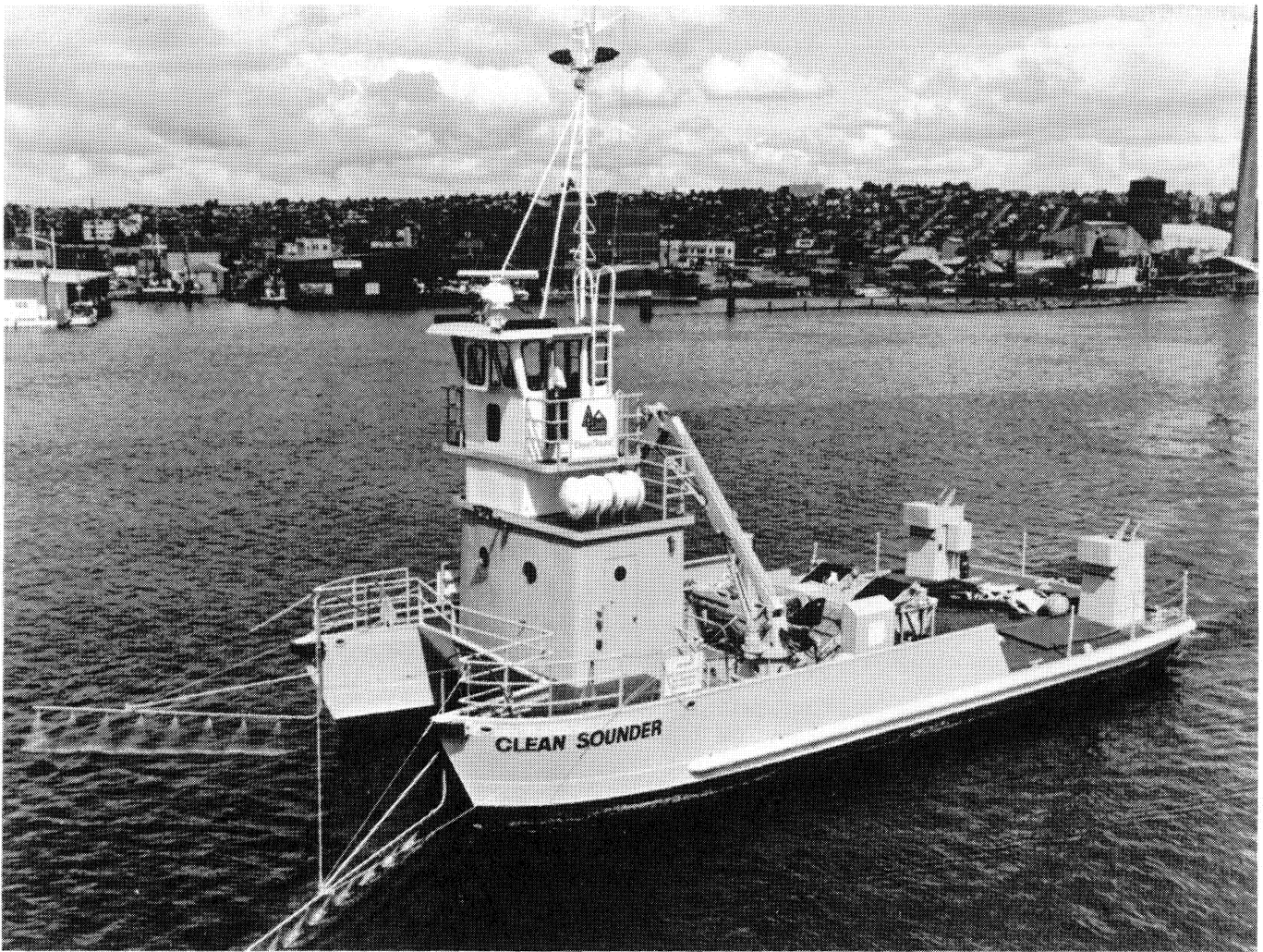
CLEAN SOUNDER undergoes operational tests. Oil-spill recovery vessel was built by Marine Construction & Design Co. of Seattle.
