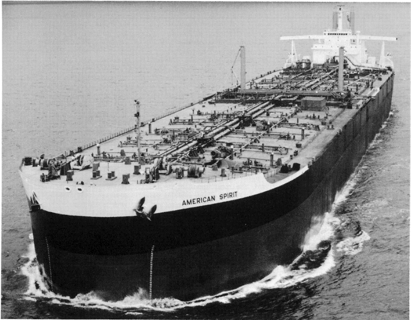
SS AMERICAN SPIRIT, first of two 265,000-dwt. tankers built at Bethlehem Steel Corp.'s Sparrows Point (Md.) Shipyard for Gulf Oil Corp., sails down Chesapeake Bay on her trials.
