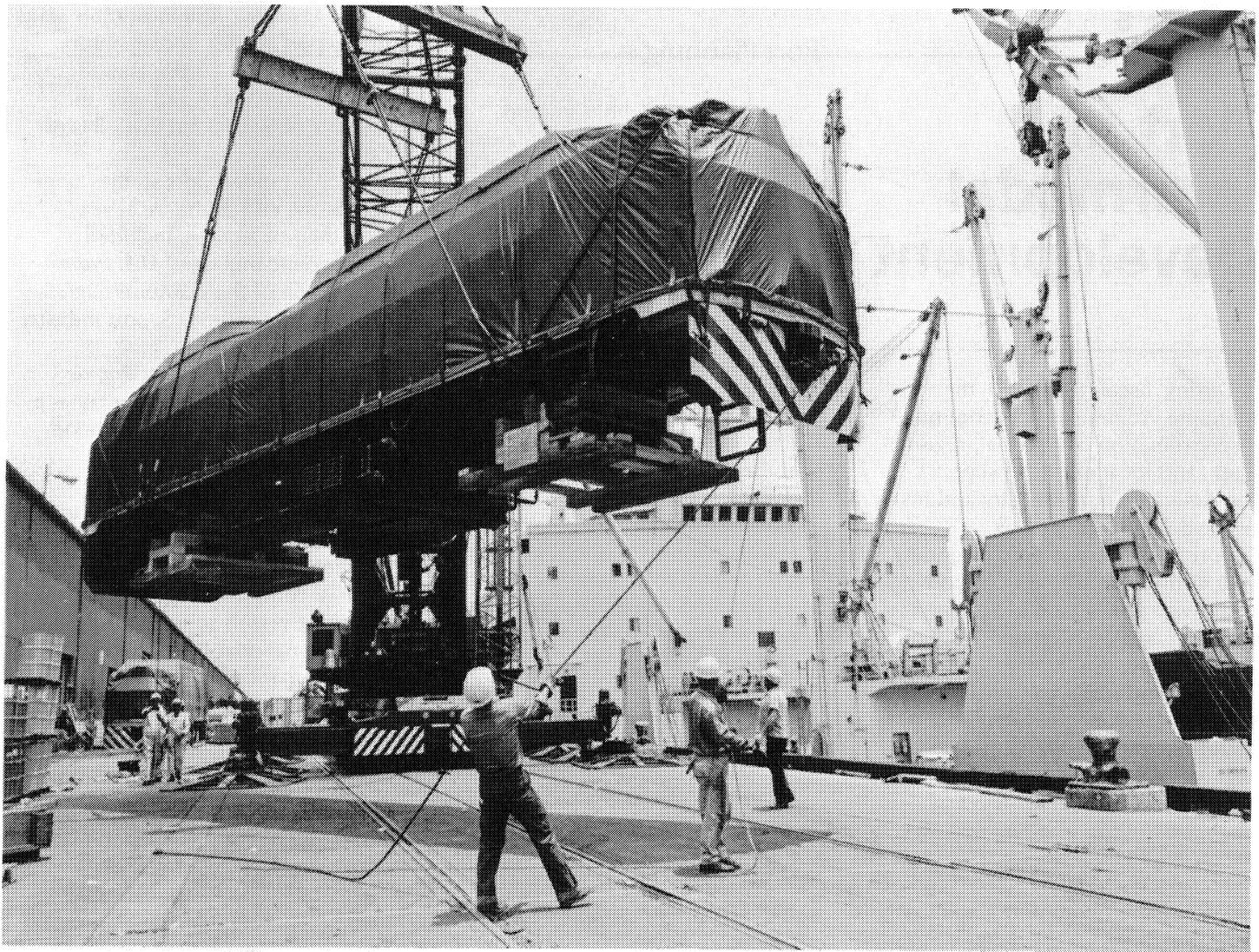
Stevedores use guide ropes to position locomotive being loaded aboard SS HOWELL LYKES at New Orleans for shipment to Peru.
