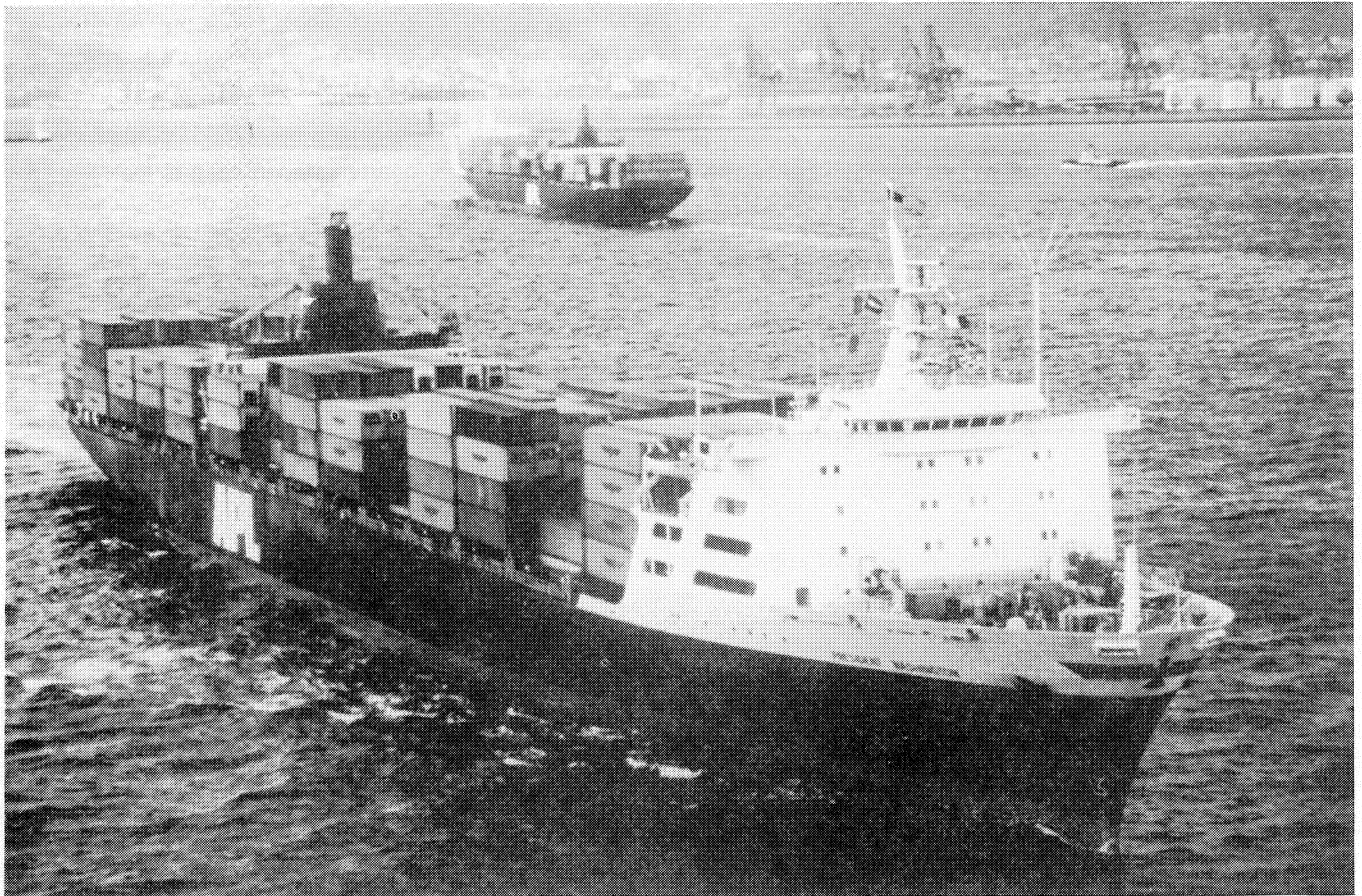
Two of American President Lines' three new containerships pass in Kobe, Japan. Built by Avondale Shipyards, Inc., and delivered in FY 1983, each vessel can carry 2,500 twenty foot containers.
