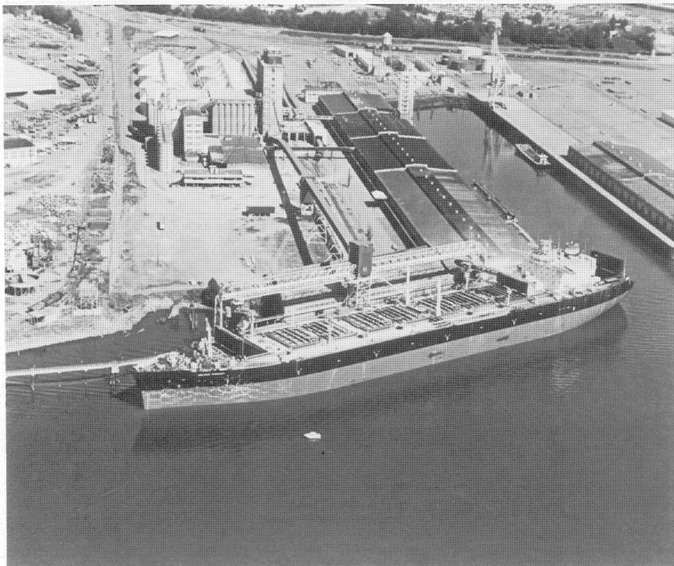
One of the two largest U.S.-flag bulk carriers, the GOLDEN PHOENIX (sistership of the JADE PHOENIX), is shown loading grain in Oregon for carriage to Egypt. Formerly a liquified natural gas carrier, the 128,000-deadweight-ton, 931-foot vessel was christened in May, 1983.
