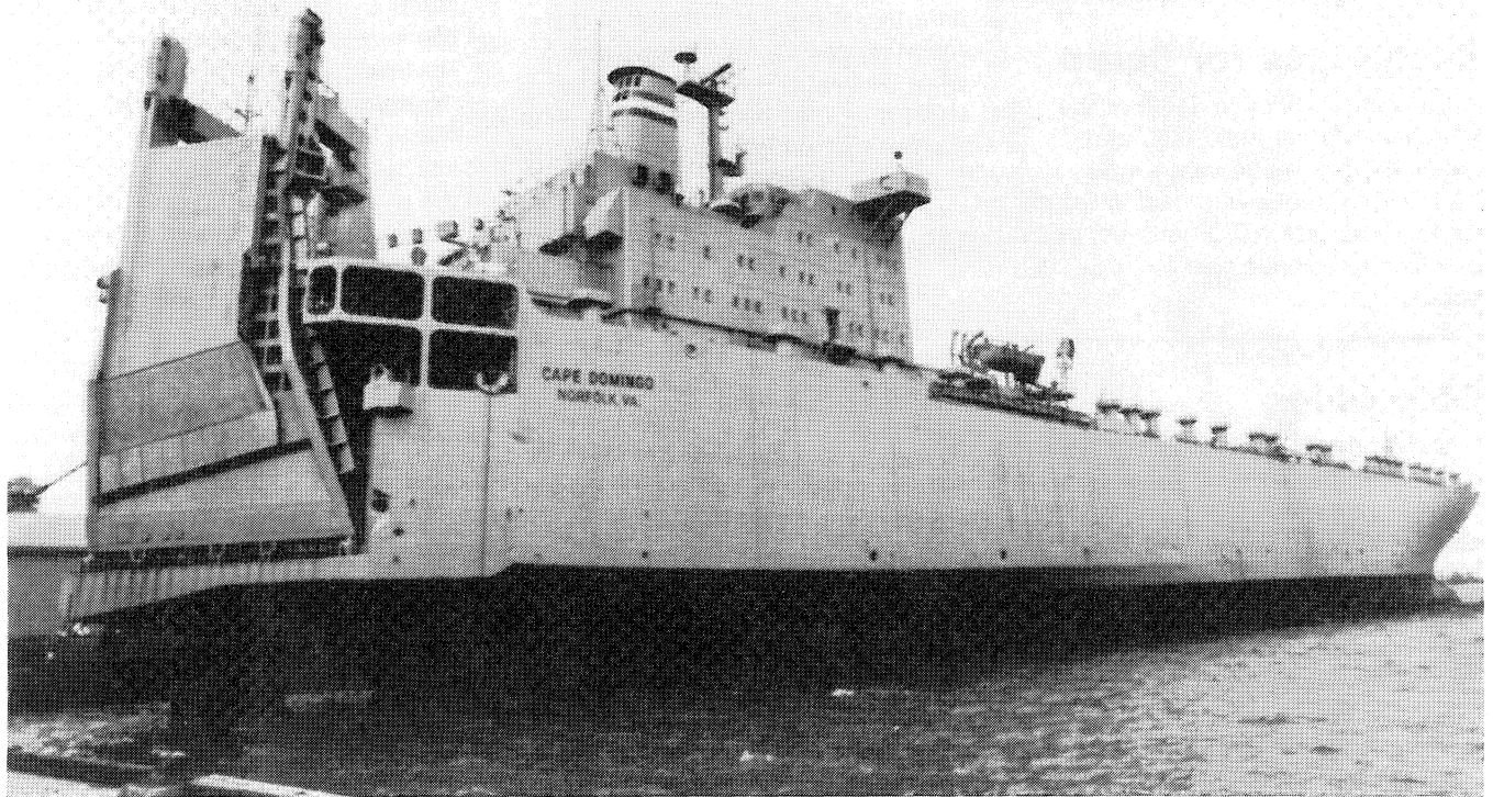
Roll-On/Roll-Off (RO/RO) vessels have a high utility as military auxiliaries. The 23,725-deadweight-ton RO/RO CAPE DOMINGO is diesel-powered with a controllable pitch propeller. It was added to the Ready Reserve Force in FY 1986.
