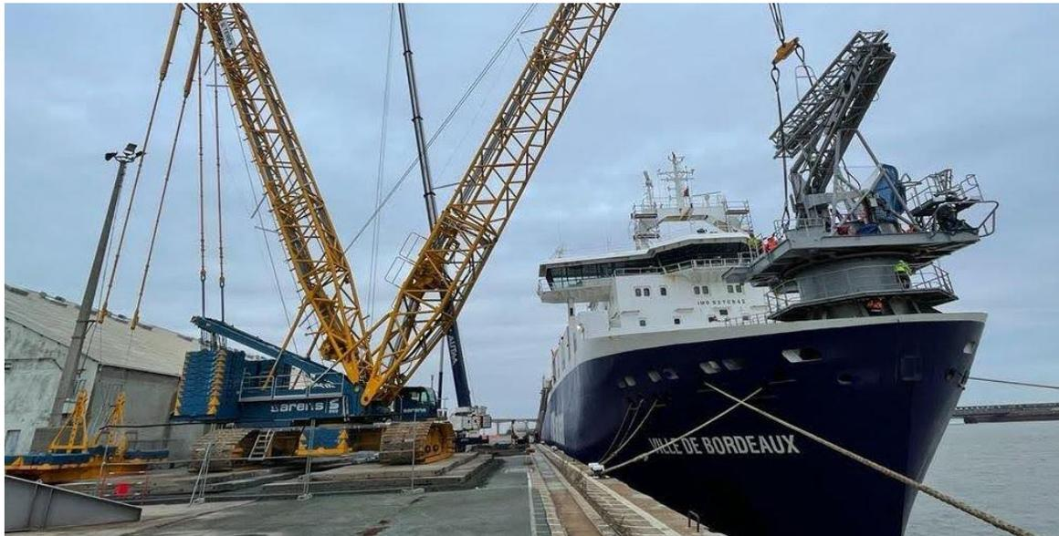
Figure 82: Seawing’s kite sail installation on *Ville de Bordeaux*, IMO no. 9270842 (source: [heavyliftnews.com](#))
