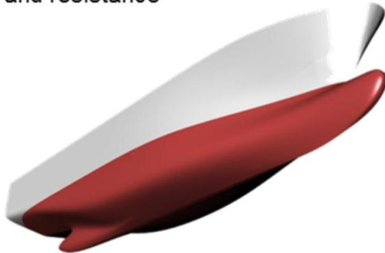
Hull optimized for build cost and resistance
