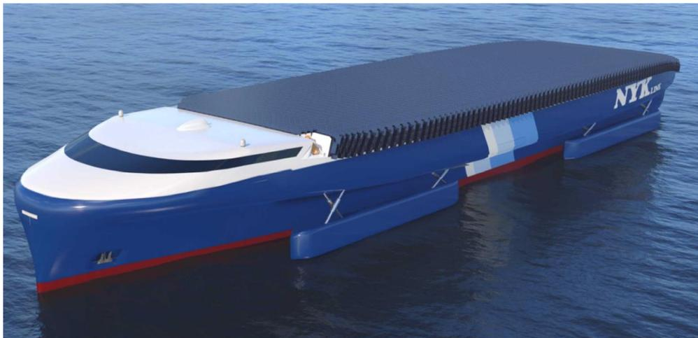
Figure 95: EcoShip 2050 concept with 9,000 m<sup>2</sup> of solar panels (source: NYK Line)
