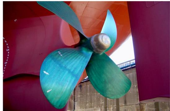
Figure 19: MAITA propeller (Source: Oshima [B9])
