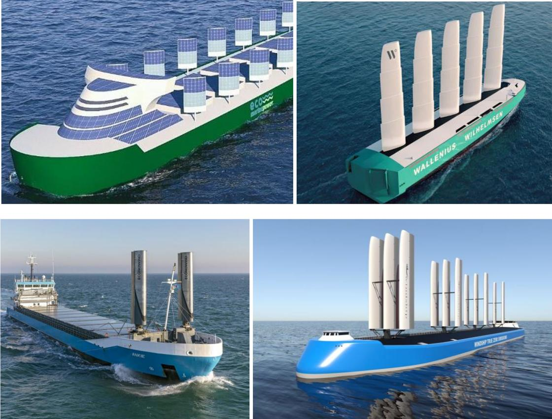
Figure 87: Various rigid wingsail technologies, clockwise from upper left: Aquarius MRE (Eco Marine Power), Orcelle Wind (Wallenius Wilhelmsen), Wingship (Wingship), and Ventifoil retrofit (Econowind)
