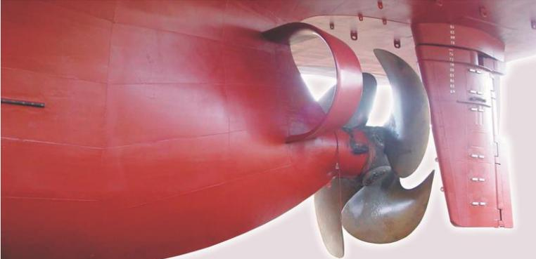
Figure 28: A Schneekluth wake equalizing duct, a type of pre-swirl duct (source: [Wartsila \[B15\]](#))
