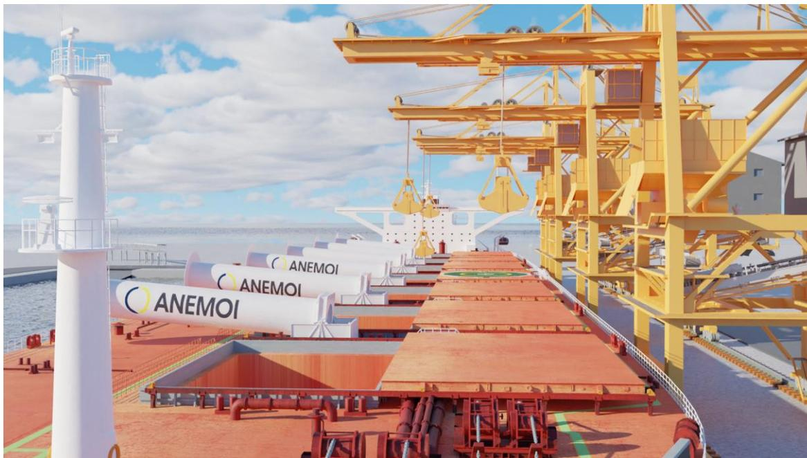
Figure 84: Rendering of Anemoi folding rotor sails on bulk carrier (source: Marine Log)
