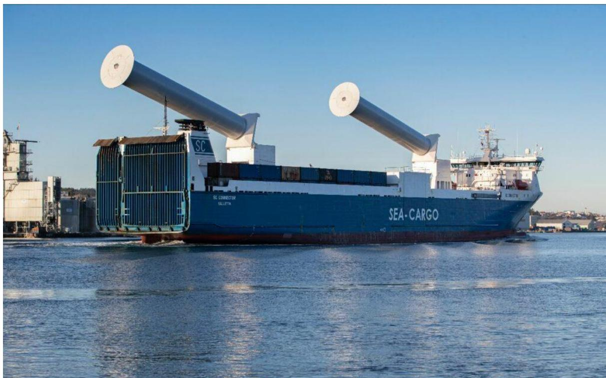
Figure 85: SC Connector RoRo with Norsepower folding rotor sails (source: Norsepower)
