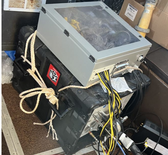
Figure 3: MKS 2030 hot-cell Fourier-transform infrared spectrometer (FTIR) and control hardware for exhaust sampling installed in the forward cabin of the Quickwater.
