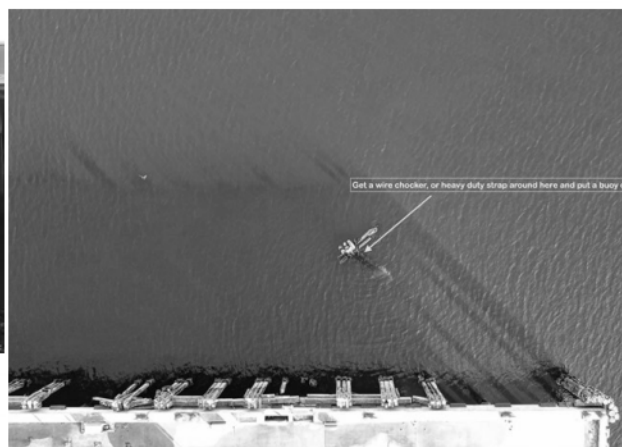
FIGURE 3 PIER FIVE PILINGS MISSING AND FLOATING
