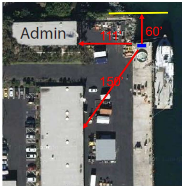
Figure 11. (Top): the SIO research vessel Robert Gordon Sproul , in port at the Nimitz Marine Facility of the SIO, San Diego, California. The blue box notionally indicates the contemplated deployment and location of the MarFC; (Bottom), distances from the MarFC unit to nearby buildings (red) and lot lines (yellow), showing compliance with NFPA 2.
