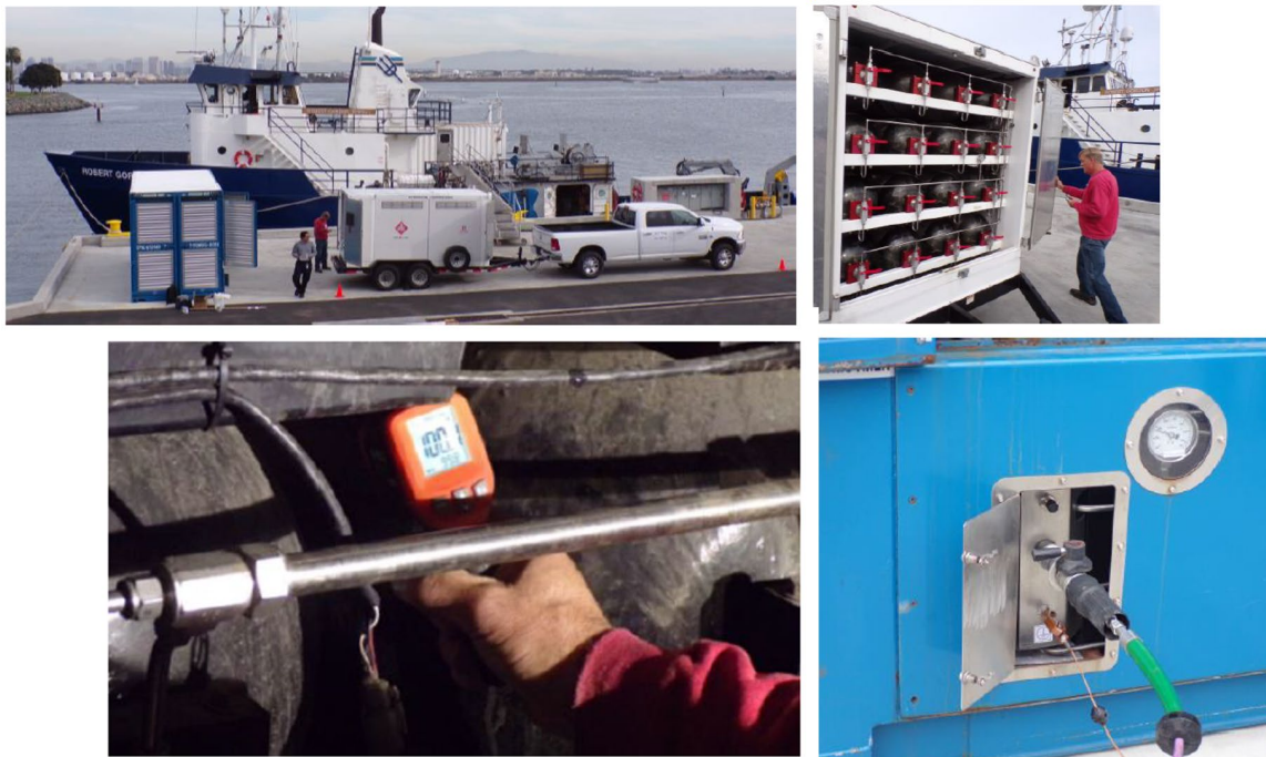
Figure 20. Clockwise from upper left: IGX H 2 refueling trailer arrives at SIO on 12/2/19; Craig Van Pelt (IGX) prepares the trailer for cascade filling; successful connection of the trailer H 2 hose (green hose) and copper grounding connection to the MarFC; the temperature of the MarFC hydrogen tanks is monitored during refueling to ensure compression-heating does not heat the tanks too much.
