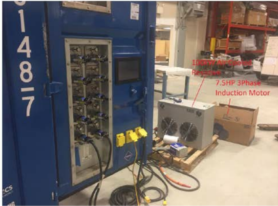
Figure 8. (L) Indoor testing of the MarFC unit at Cummins/Hydrogenics after system repair and upgrade; (R) outdoor testing of the MarFC unit in cold weather at the Cummins/Hydrogenics site in Mississauga, Ontario, Canada, December 2017.
