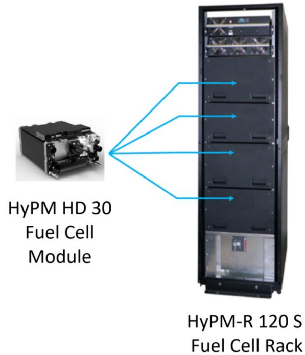
Figure 3: Hydrogenics HyPM-R 120S fuel rack (right) assembled from four HyPM HD 30 33 kW PEM fuel cell modules (left). Photo courtesy of Ryan Sookhoo, Cummins.
