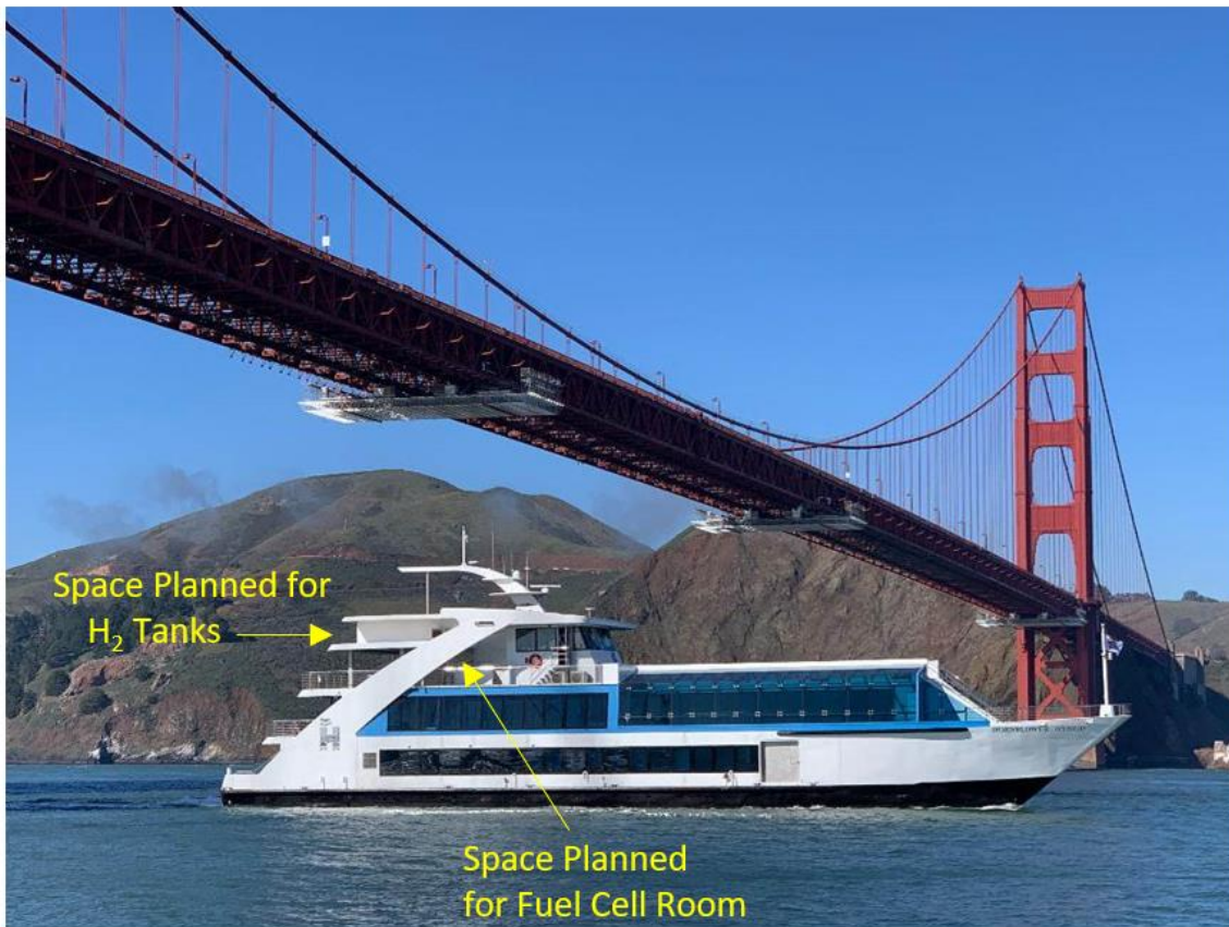
Figure A: The New York Hornblower Hybrid sailing underneath the Golden Gate to its new home on the San Francisco Bay. Indicated are the storage spaces allotted to H 2 tanks and the Fuel Cell Room designed to house PEM fuel cells.
