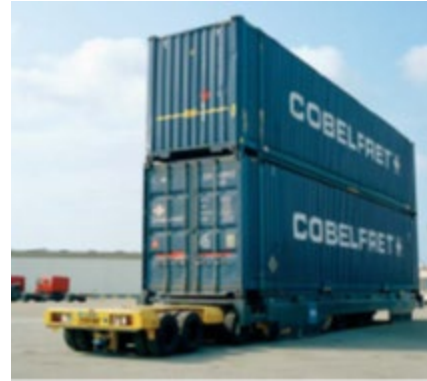
Cassette for multi-length containers (40'/45') on special trailer
