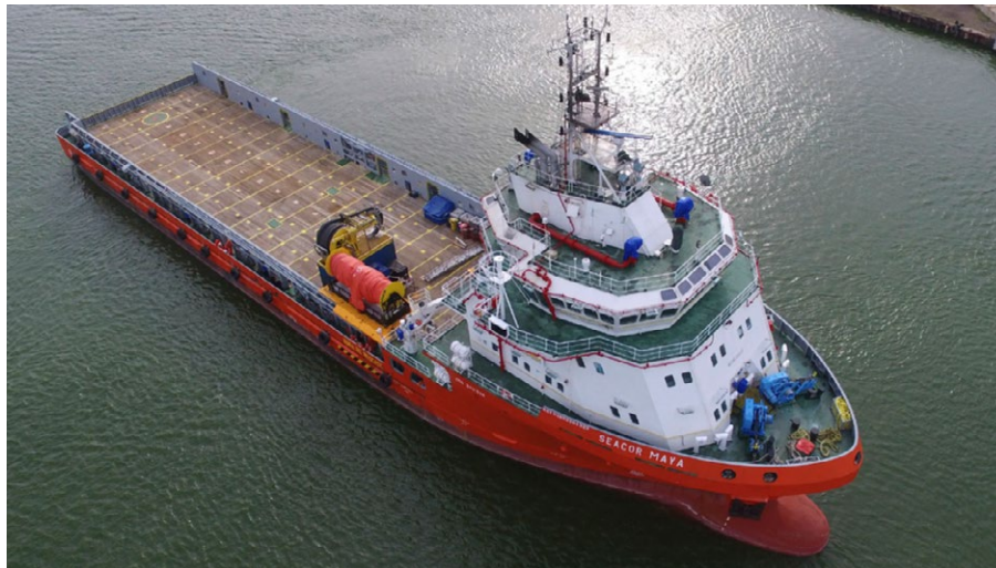
Figure 35: Dynamically Positioned Diesel-Electric Vessel, OSV SEACOR MAYA
