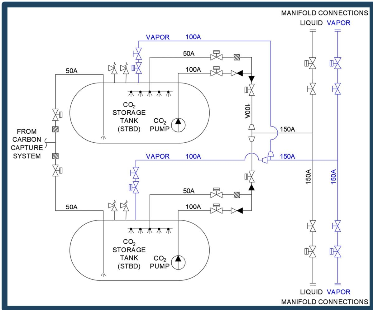
Figure 8: CO<sub>2</sub> Tank and Offloading Schematic
