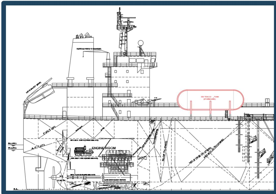
Figure 7. Elevation View Showing CO<sub>2</sub> Storage Tank Location
