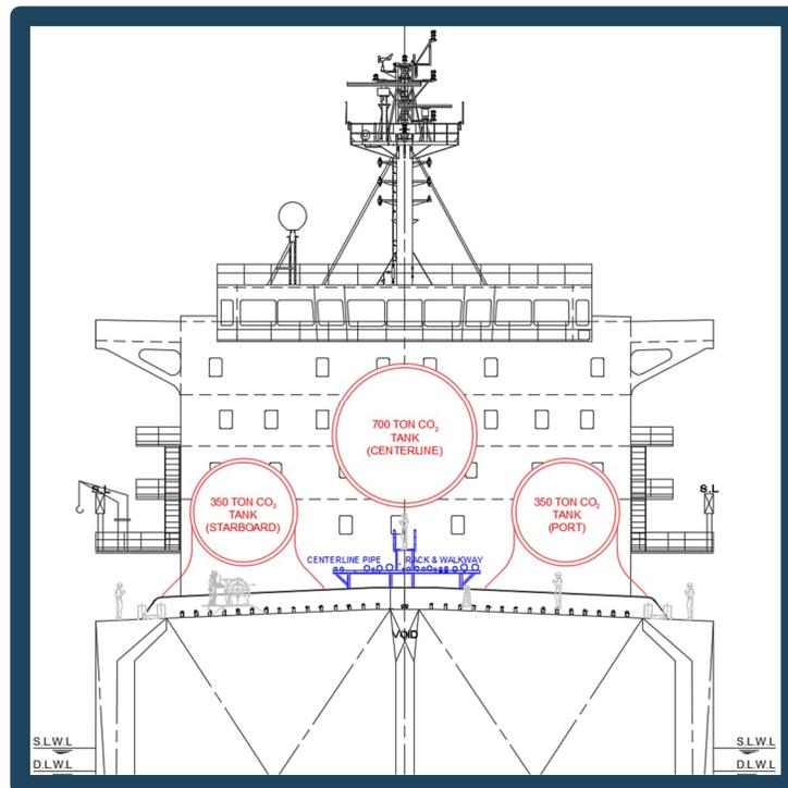
Figure 6. Section View Showing Potential CO<sub>2</sub> Storage Tank Locations
