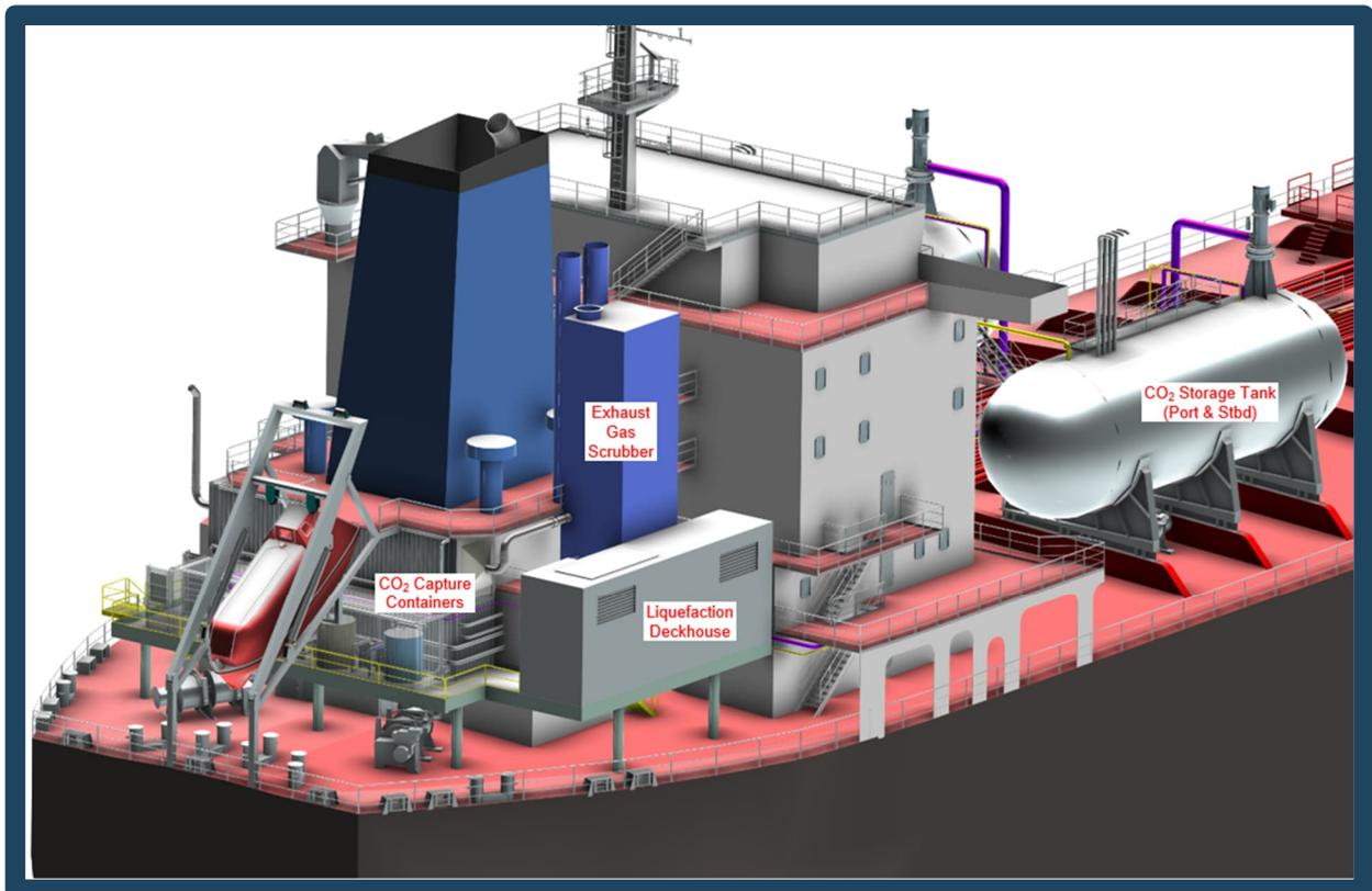
Figure 4. Conditioning and Capture equipment locations for 1 ton per hour capacity.
