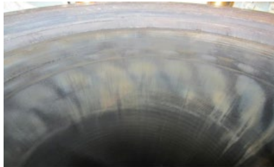
Figure 6.1. Upper cylinder liner after a sea trial showing white patches indicative of early cold corrosion. Photograph courtesy of MAN Energy Solutions., 2013.
