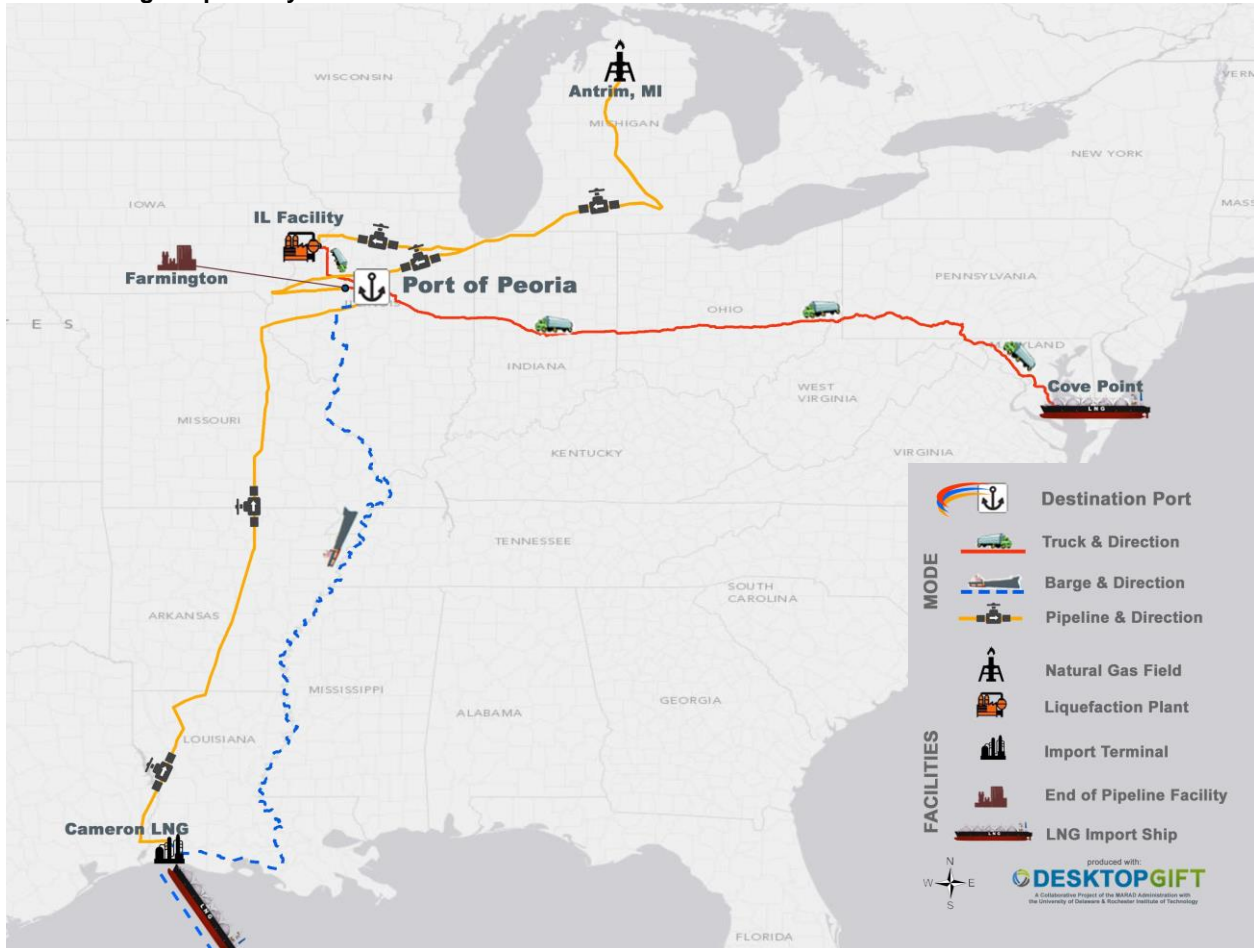
Figure 22 Depiction of various fuel pathways for the Peoria end of the Inland Case showing transportation modes along the pathway network
