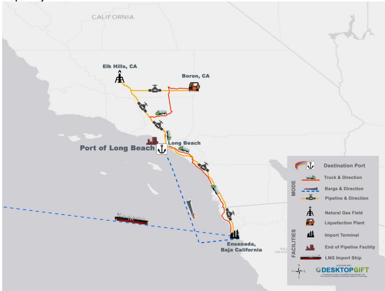
Figure 4 Depiction of various fuel pathways for the West Coast Case showing transportation modes along the pathway network
