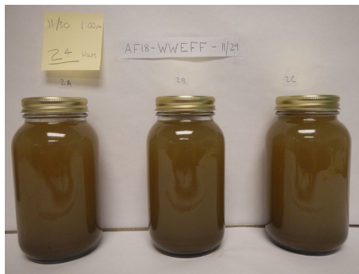
Figure 3-8 Wedge Wire Screen Effluent After 24 Hours of Settling
