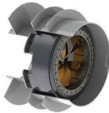
Figure 11 Rim thruster (Schottel SRT)
