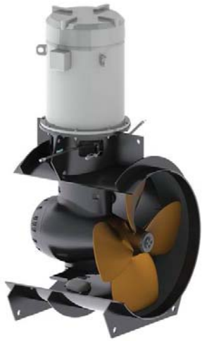
Figure 10 Electric motor driven tunnel thruster (Schottel STT)
