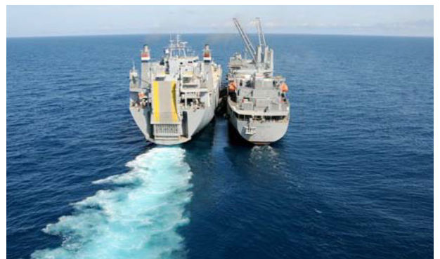
FLICKERTALE STATE (right) and the CAPE TEXAS (left) – photo courtesy the U.S. Navy The vessels are moored and fendered ‘skin-to-skin’ to test advanced crane control technologies.
