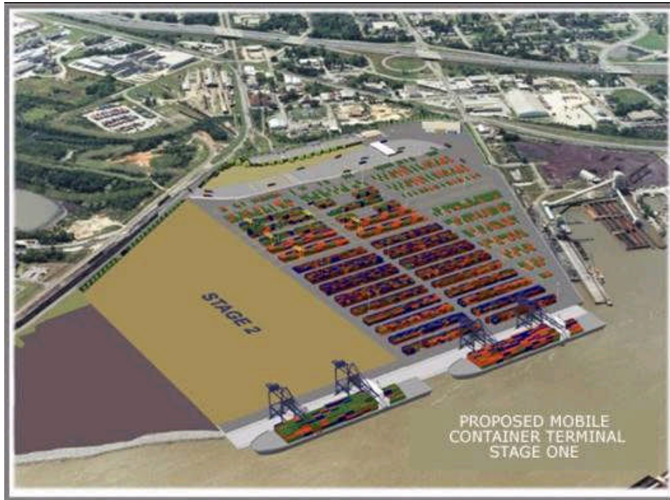
Exhibit 48: Typical Two-Berth/Four-Crane Terminal
